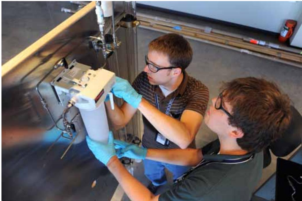
The current first phase involves stress-testing the metallic alloys in a machine at CAES that simulates the high-temperature water in the nation's nuclear reactors. Jackson, INL's Sebastien Teysseire and others on the team (including researchers from MIT and other universities and national laboratories) are conducting the tests to monitor when cracks develop and how fast they grow.
