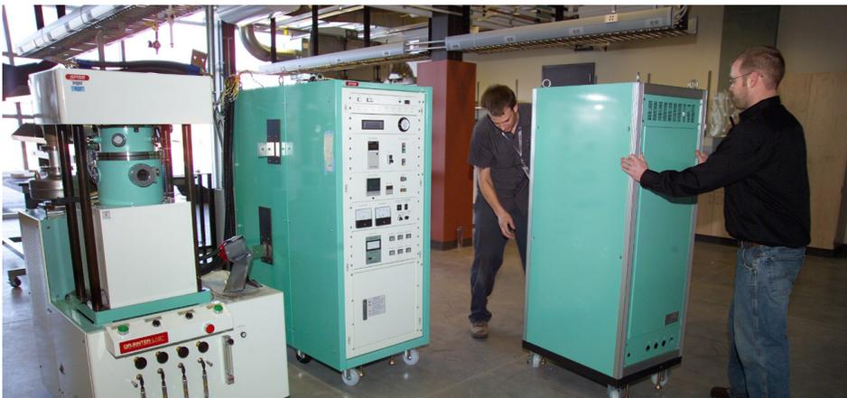
Vendors moved Boise State University's spark plasma sintering system into CAES' materials laboratory in April. The device allows CAES researchers to combine metals, ceramics and other hard-to-process materials. It will play a key role in the research conducted at the Radioactive Materials Processing Center (RAMP-C).
