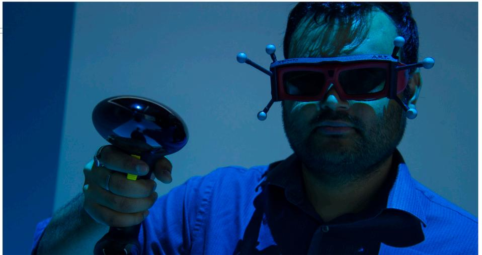
*The updated CAVE uses rear digital projection projectors to display computer graphics on three walls and the floor, which can be viewed through stereoscopic glasses and manipulated with a wand.*
